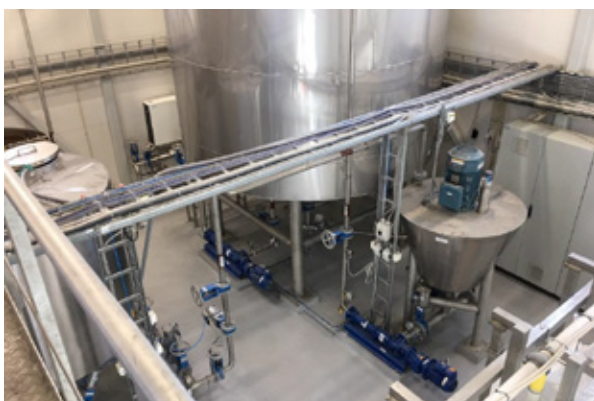
Fig. 9 Inside plant showing dissolver to he right
